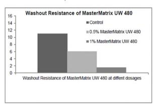
Cement content of 385 kg/m $^3$ , water-cementitious material ratio 0.49; slump 100  $\pm$  15mm; non airentrained.
